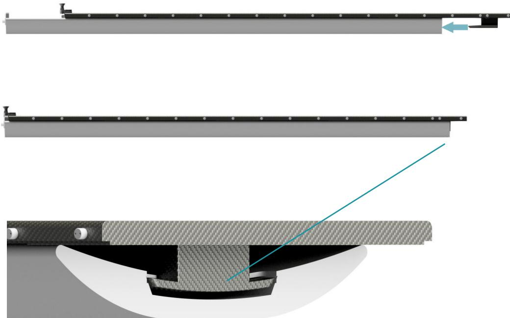
IV. Check if the indexing plungers are stuck in the corresponding holes of the caudal plate. To release the CouchTop, pull the plungers.
