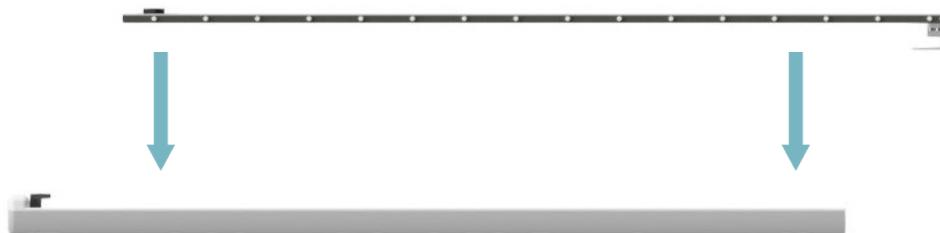
IV. Slide the CouchTop towards the caudal end of the cradle. Take care that the CouchTop aperture fits the holding block.
