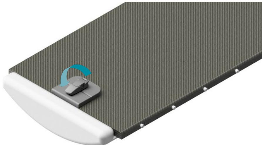
VII. Tighten the four screws from step three, located at the cranial side.
