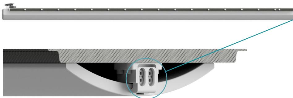
VI. Turn the latch caudal to lock the CouchTop in longitudinal direction. Check if the latch can close properly without any play in longitudinal direction after locking. If necessary, the latch block can be adjusted in longitudinal position to remove any longitudinal play.
