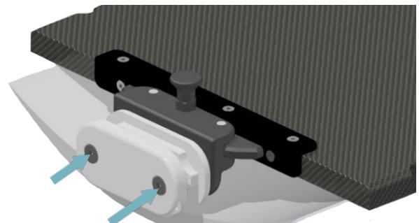
II. At the cranial end of the CouchTop, loosen the four screws of the spoon (circled) with an Allen key.
