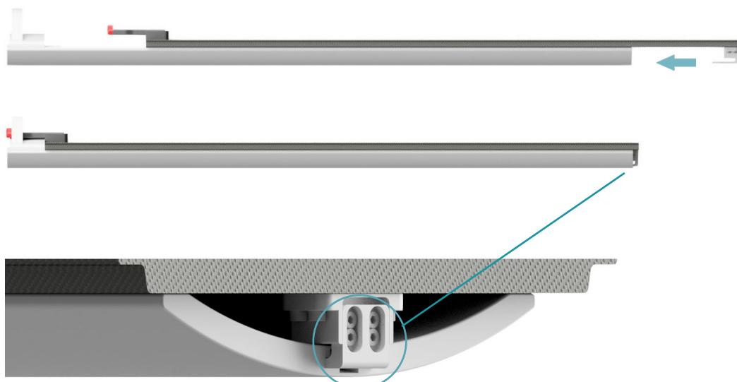
V. If needed, adjust the CT lockers to eliminate play in longitudinal direction. Turn the clamps lateral, place them against the caudal arch and tighten the screws.
