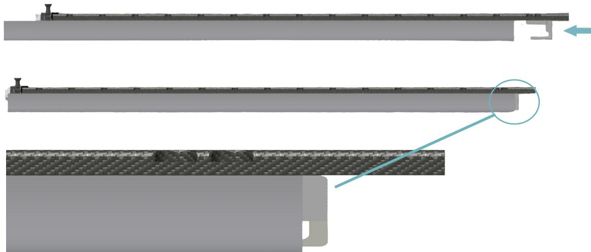
IV. Now that the caudal end is approaching the caudal block, pull the indexing plunger knob and push the CouchTop against the caudal block. Once in place, release the indexing plunger knob to secure the CouchTop to the cradle.
