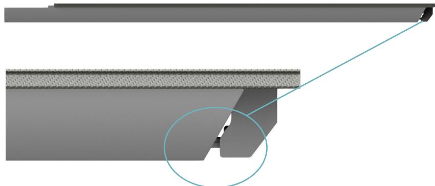
V. Check if the indexing plunger (circled) is fixed in the Caudal block of the CouchTop. If needed, adjust the Caudal block in longitudinal direction and/or the height of the indexing plunger.
