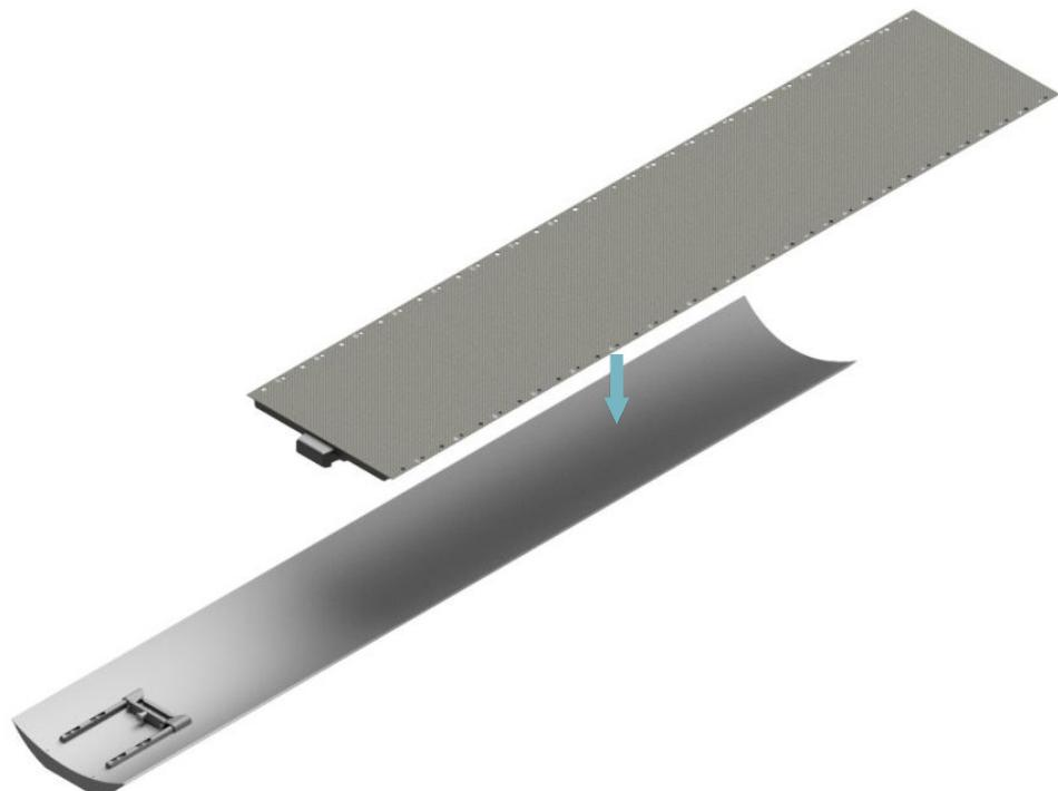
IV. Slide the CouchTop towards the caudal end of the cradle until its lays flat against the caudal cradle block. Make sure that the cranial position block slides into the cradle.
