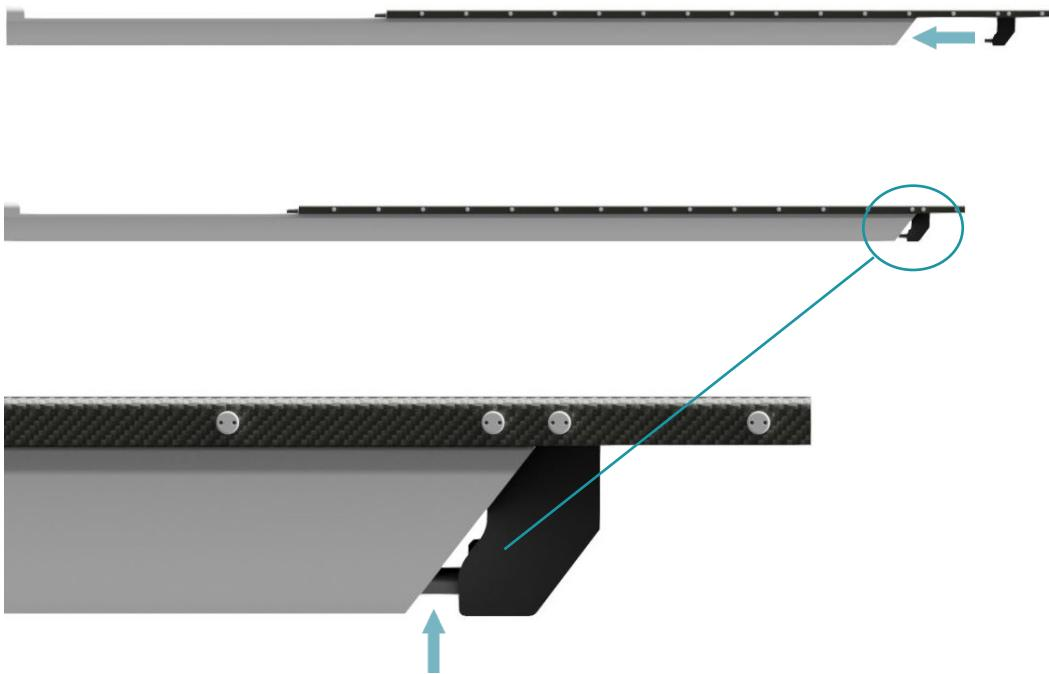
V. Check if the indexing plunger (circled) is fixed in the caudal block of the CouchTop. If needed, adjust the indexing plunger in height by using an Allen key to loosen and tighten the screws of the caudal cradle plate.
