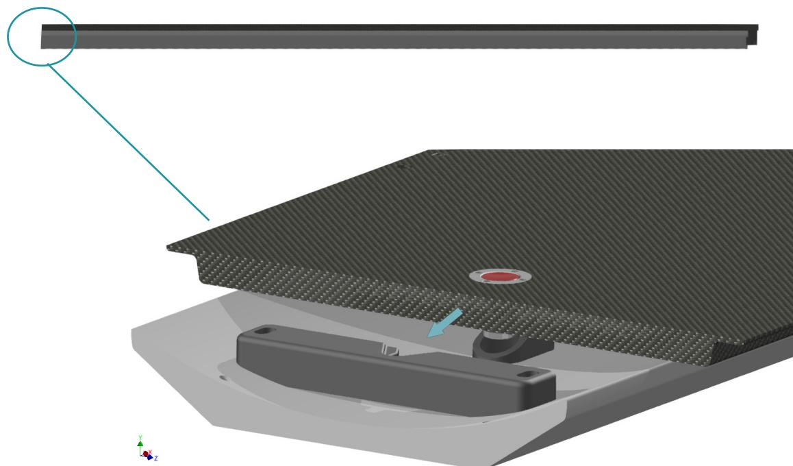
II. As the CouchTop slides into the caudal block, the red button will be pushed upwards.
