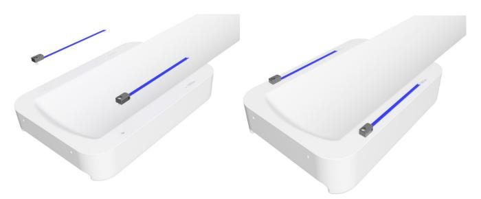
II. Be aware of a left and right version of the guidestrip. Make sure that the hole for the indexing plunger points towards the lateral direction. Tighten the set screw with an Allen key until the caudal block is secured to the cradle.
