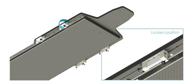
V. Tighten the black adjusting knobs to fix the couch. With the Allen key, turn the M4 bolts to lock the black adjusting knobs.
