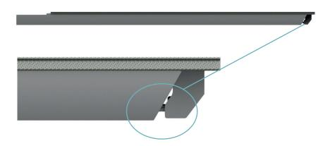
V. Check if the indexing plunger (circled) is fixed in the Caudal block of the CouchTop. If needed, adjust the Caudal block in longitudinal direction and/or the height of the indexing plunger.
