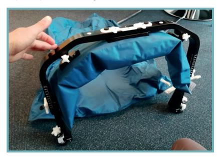
V. After treatment, detach the Vacuum Cushion from the Secure Arch by slide the white locking plate to the left and turn the aforementioned star shaped locking knobs counterclockwise.
